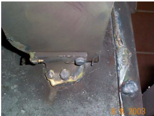
You don't want your ACB cassette to end up like this after a plug-in retro-fit ACB.....
